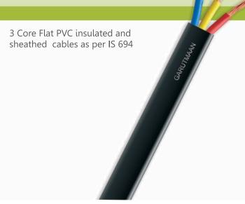
"Garutmaan" PVC insulated and sheathed 3 Core Flat cables, conforming to IS 694, are manufactured using high conductivity, electrolytic grade, bright, plain annealed copper conductors.
